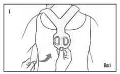
1. Position the D-ring pad in the center of the back. Place straps over each shoulder.
